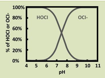
Two Methods for Optimizing pH of Free Chlorine Solution
